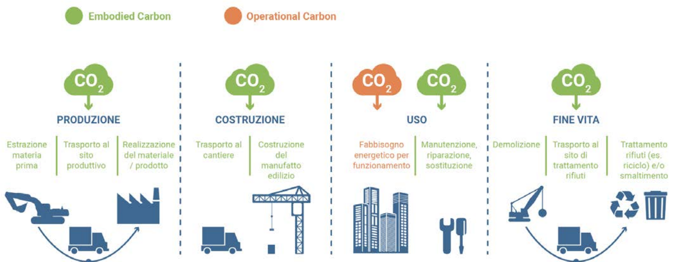
Figura 1.2 – Emissioni di CO 2 associate al ciclo di vita di un manufatto edilizio (elaborazione degli autori su fonte: BPIE (Buildings Performance Institute Europe) (2021). Whole-life carbon: challenges and solutions for highly efficient and climate-neutral buildings. https://www.bpie.eu/publication/whole-life-carbon-challenges-and-solutions-for-highly-efficient-and-climate-neutral-buildings/
